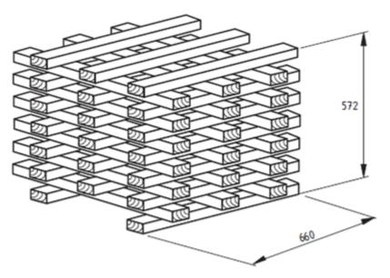
Figure A.1 - A typical wooden crib for the semi-natural fire exposure test
